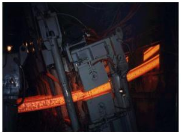
Figure 8 - Straightener Withdrawal Units for Strand Unbending
