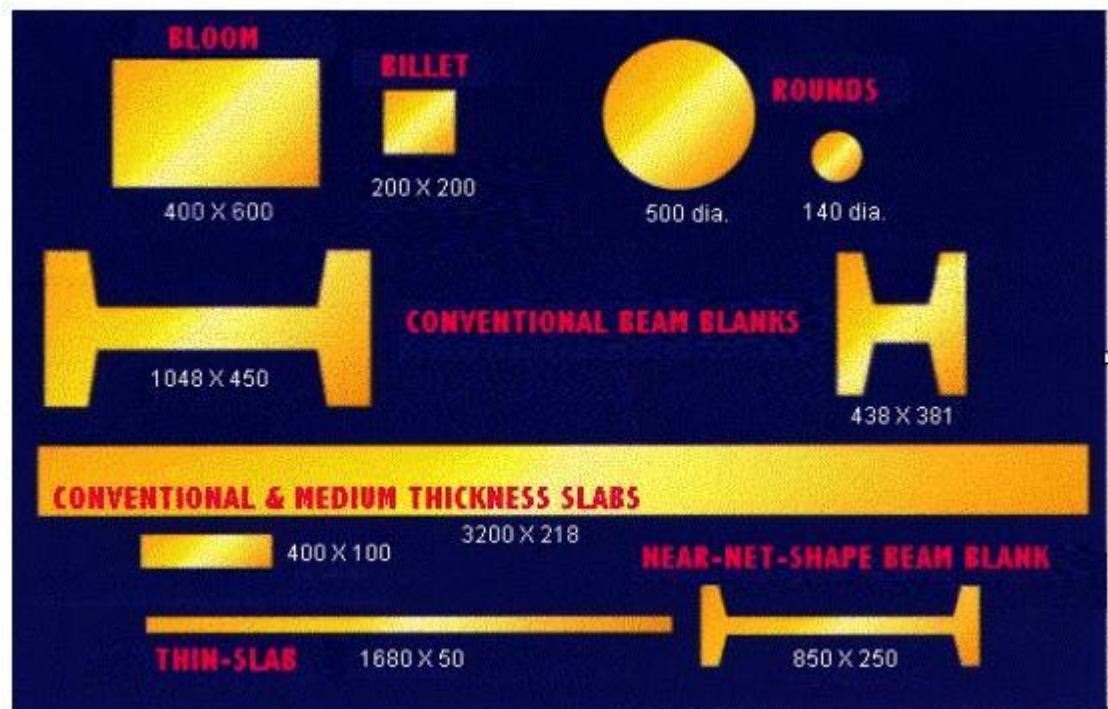
Figure 4 - Continuous Cast Shapes (sizes in millimeters)
